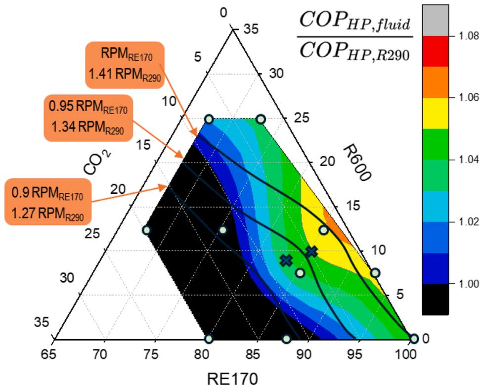
Fig. 12. Relative  $COP_{HP}$  as function of mass percentage of components.
