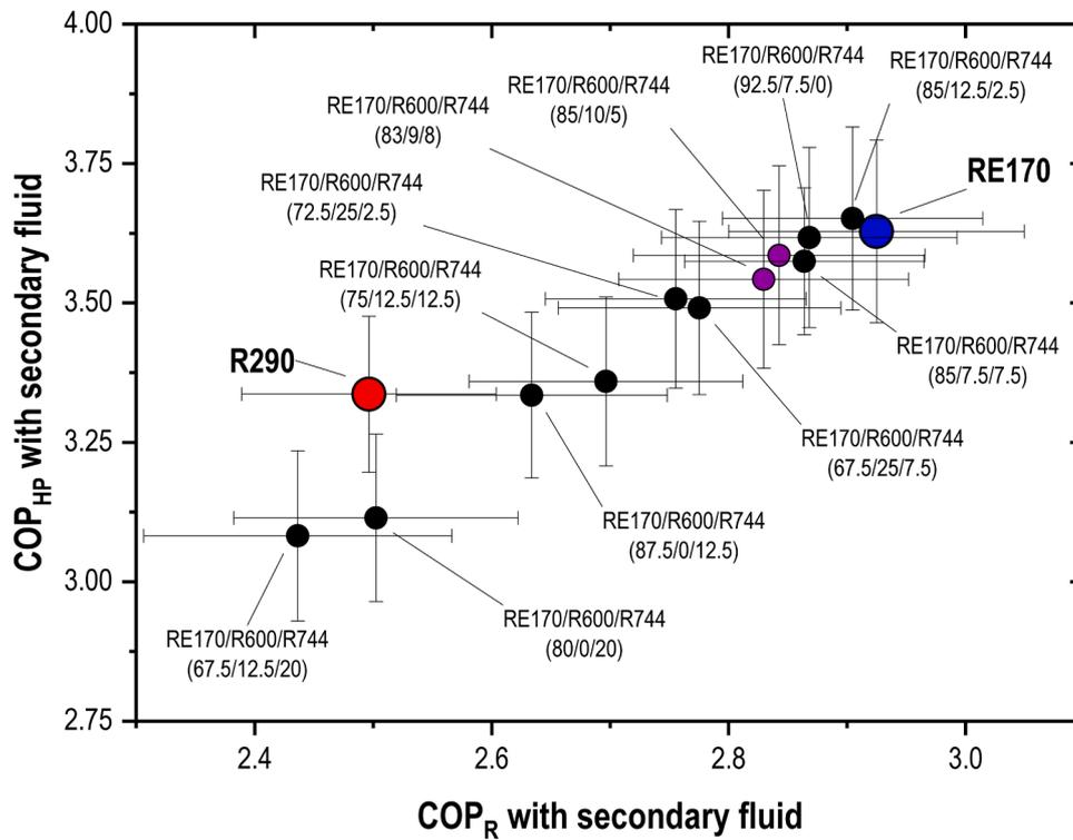
Fig. 7. COP<sub>HP</sub> vs. COP<sub>R</sub> at fixed cooling capacity test conditions.
