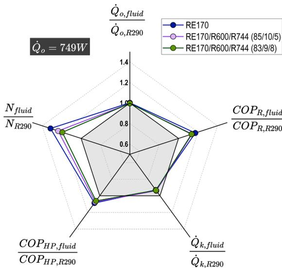
Fig. 14. Relative main parameters in relation to R290 in fixed cooling capacity test.
