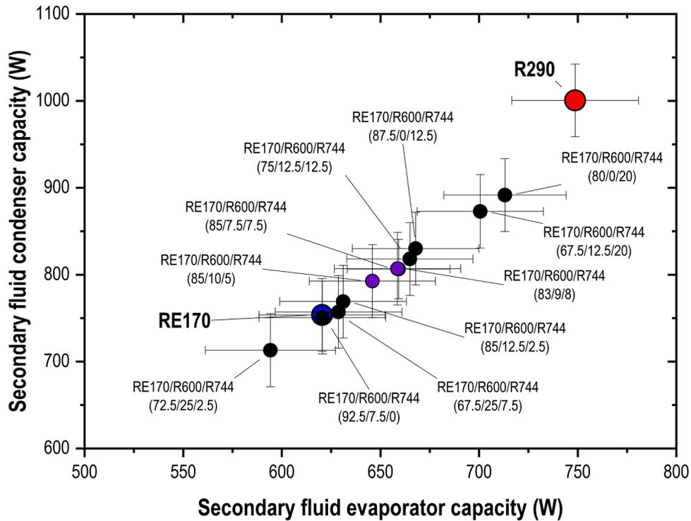
Fig. 6. Q<sub>k</sub> vs. Q<sub>o</sub> at drop-in test conditions.
