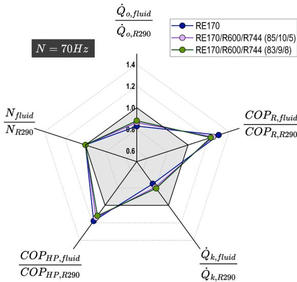
Fig. 13. Relative main parameters in relation to R290 in drop-in test.
