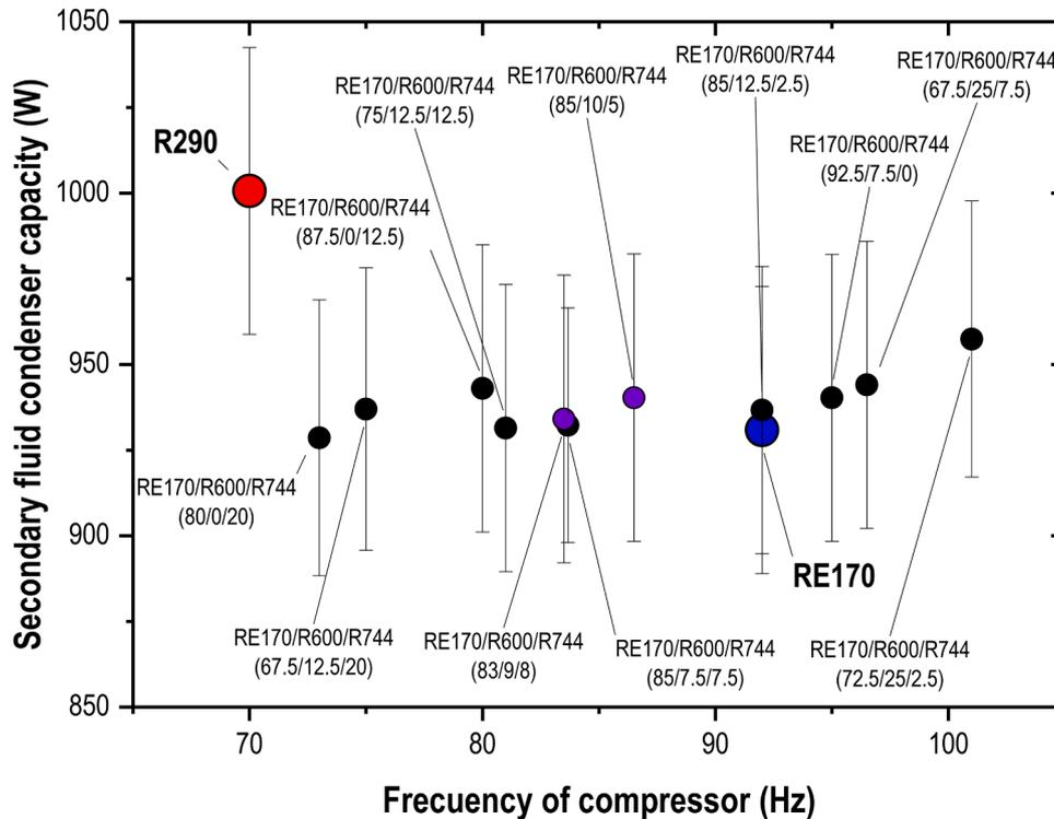
Fig. 8. Q<sub>k</sub> vs. compressor frequency at fixed cooling capacity test conditions.
