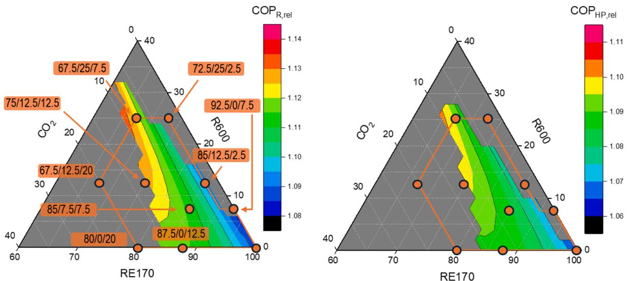
Fig. 2.  $COP_{R,rel}$  (left) and  $COP_{HP,rel}$  of mixtures respect to R290. Points to be tested experimentally.
