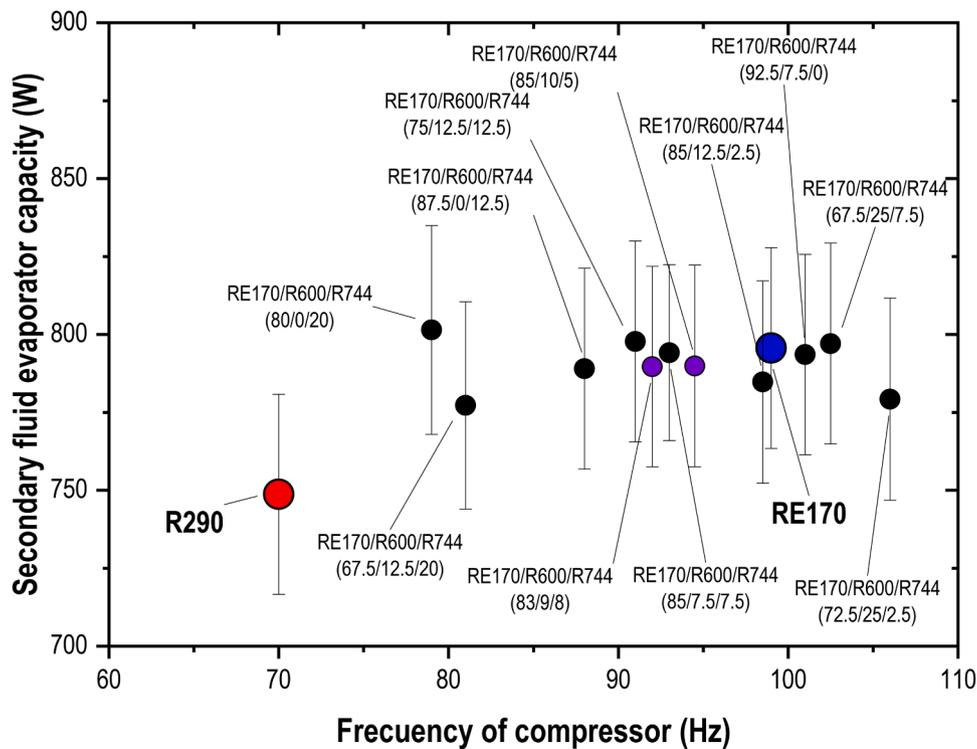
Fig. 10. Q<sub>o</sub> vs. compressor frequency at fixed heating capacity test conditions.
