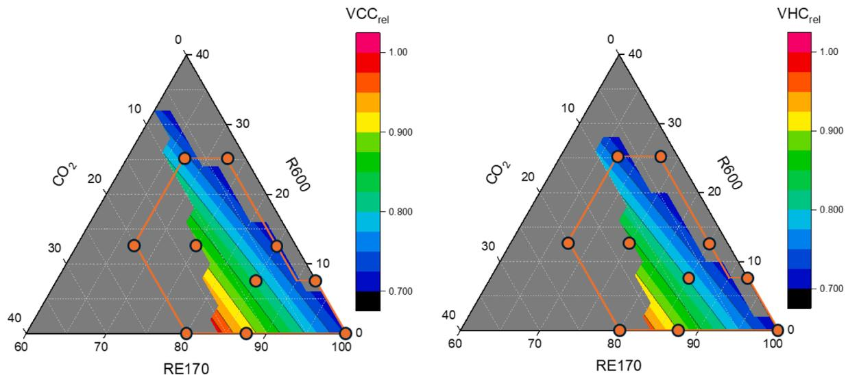
Fig. 3.  $VCC_{rel}$  (left) and  $VHC_{rel}$  (right) of mixtures respect R290.
