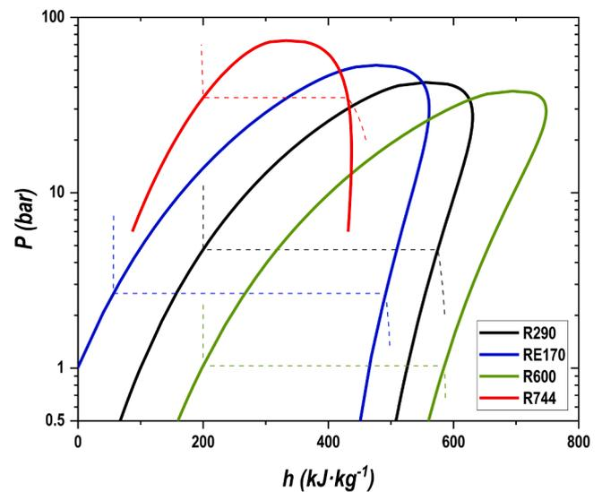
**Fig. 1.** Pressure enthalpy diagram of pure components and 0 °C isotherm.
