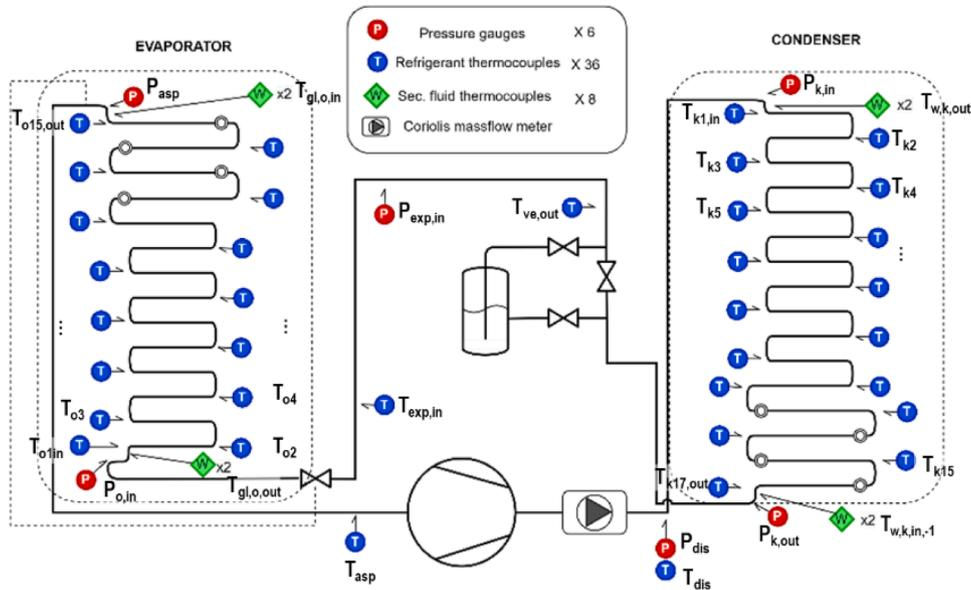
Fig. 4. Scheme of the test bench and allocation of measurement devices.
