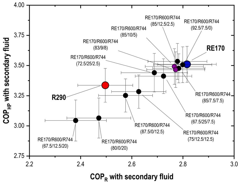
Fig. 9. COP<sub>HP</sub> vs. COP<sub>R</sub> at fixed heating capacity test conditions.
