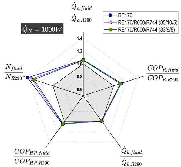
Fig. 15. Relative main parameters in relation to R290 in fixed heating capacity test.
