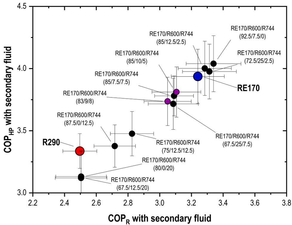
Fig. 5. COP<sub>HP</sub> vs. COP<sub>R</sub> at drop-in test conditions.
