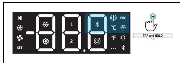
Figure 6-3 - CC200 Case Display Unlock
