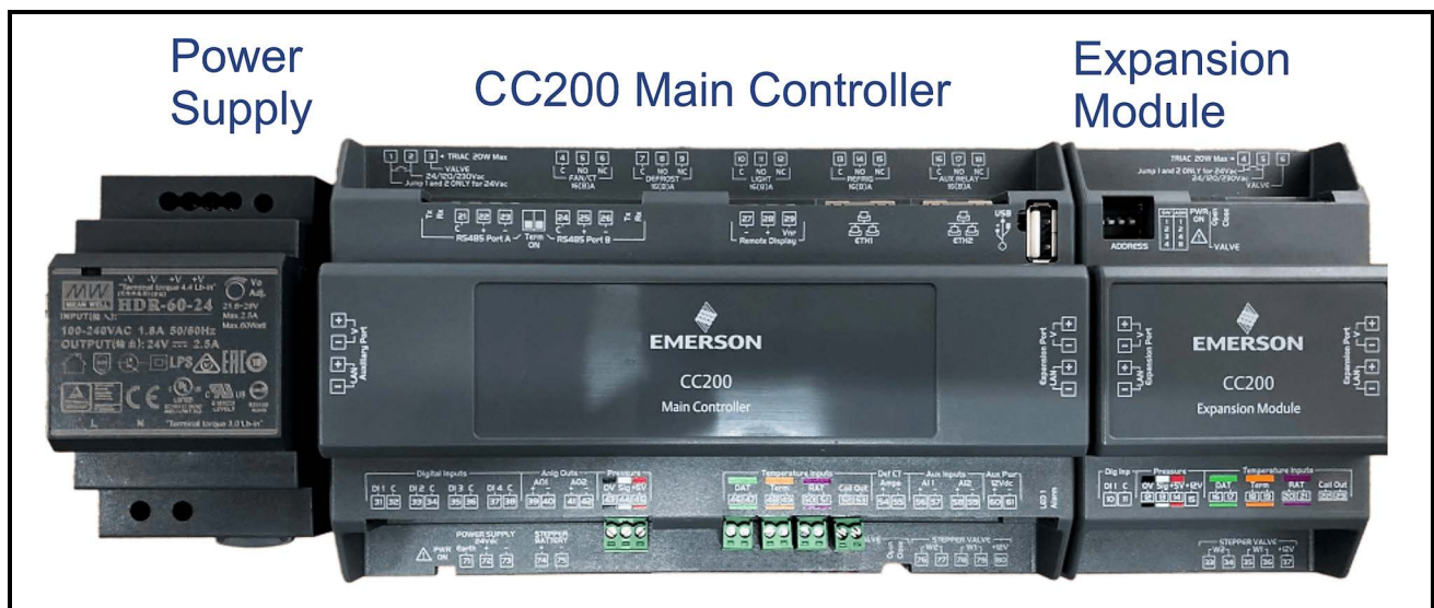
Figure 1-1 - Case Controller 200 (CC200)
